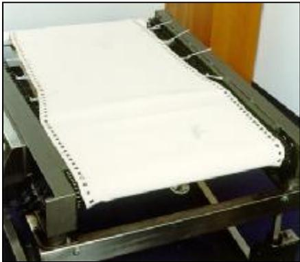
11. To avoid excessive local belt loading, fix the belt to the chain with Cable Ties. Use approximately 4 cable ties on each side spaced equally along the length of the belt. Secure each cable tie with a nut and washer. If the cable tie is not long enough, two can be looped together.
