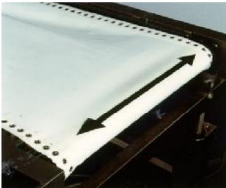
9. Care must be taken to ensure that the separating belt is installed parallel with the chain attachment studs exactly in-line and parallel to the axis of the end rollers.
