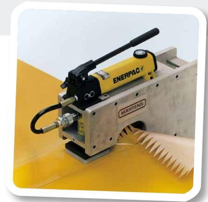
The 1st punching process can begin, i.e. close the rotary valve and bring the unit to pressure by operating the hydraulic pump.
