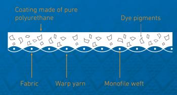
2. Cross-section of PU conveyor belt made of pure PU without pigments
