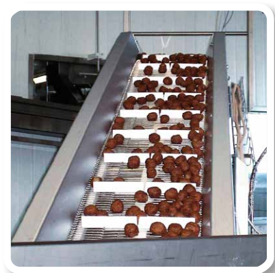
Rod network belt with carriers in operation (inclined conveying of meat balls)
