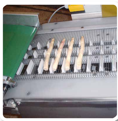
Rod network belt with individual carriers in operation (washing and cutting machine for asparagus)
